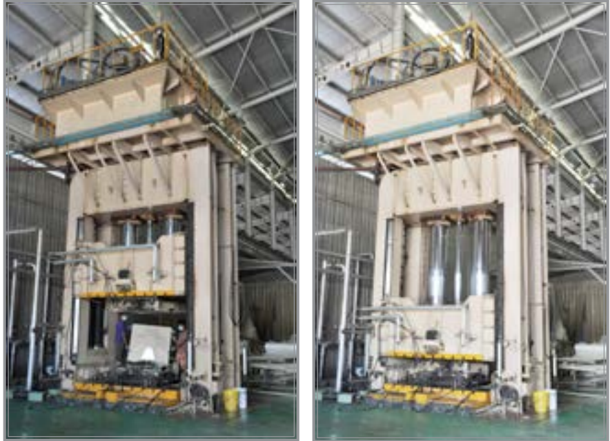
State-of-the-art 600 metric tonnes hydraulic press, one of the country's biggest units for FRP water tank panel moulding.
